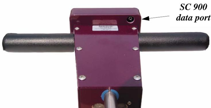
The data port on the underside of the SC 900 meter (shown above) can be accessed by removing the plastic screw. It is through this port that the meter is connected to either a PC or to a GPS unit.
